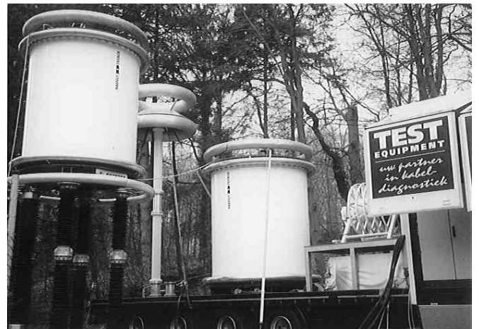
Figure 3: Test set-up to reactors in series ( 2S1P)
