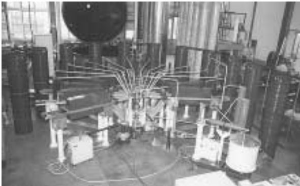
Fig. 5 Test equipment for "Operating Duty Test" according /1/
