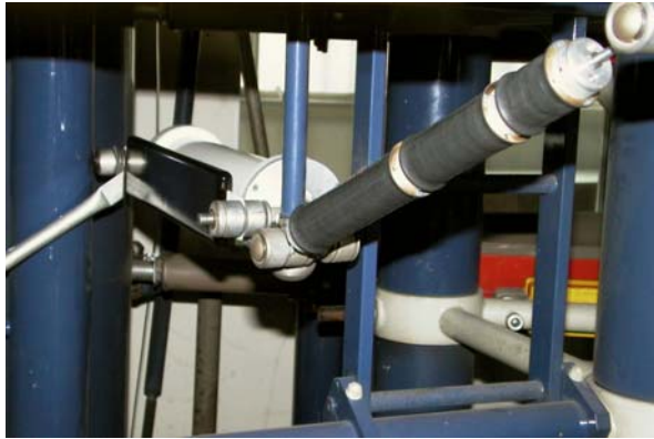
Fig. 5: Example for an internal series compensation within a Haefely generator
