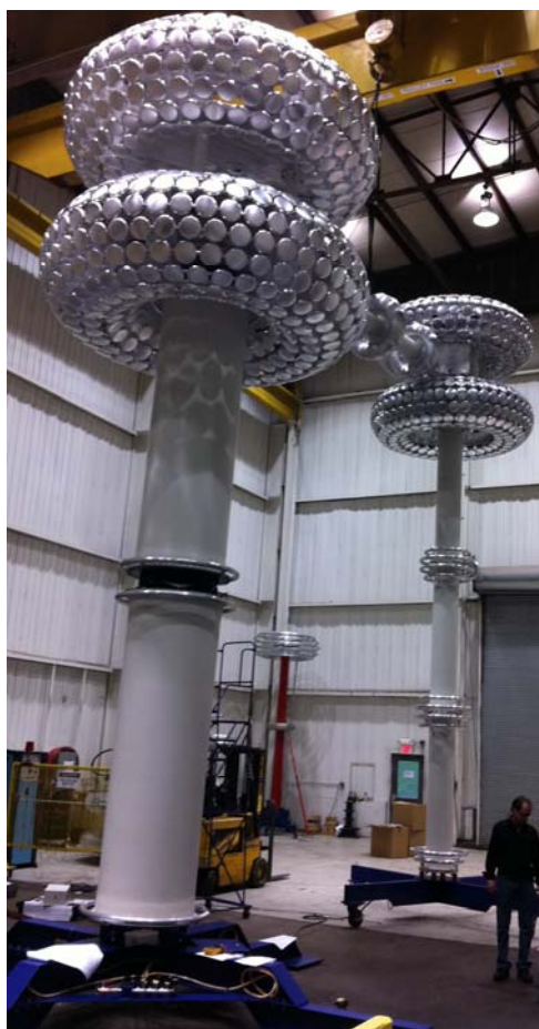
Fig. 2: Stacked voltage doubler system for 1.2 MV during erection
